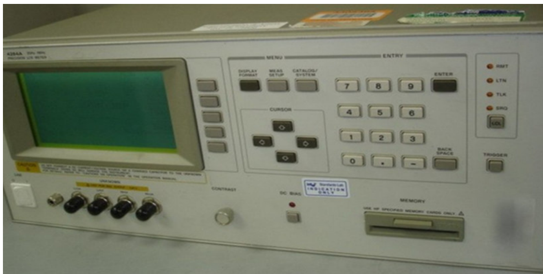
Figure (3-8) LCR meter
