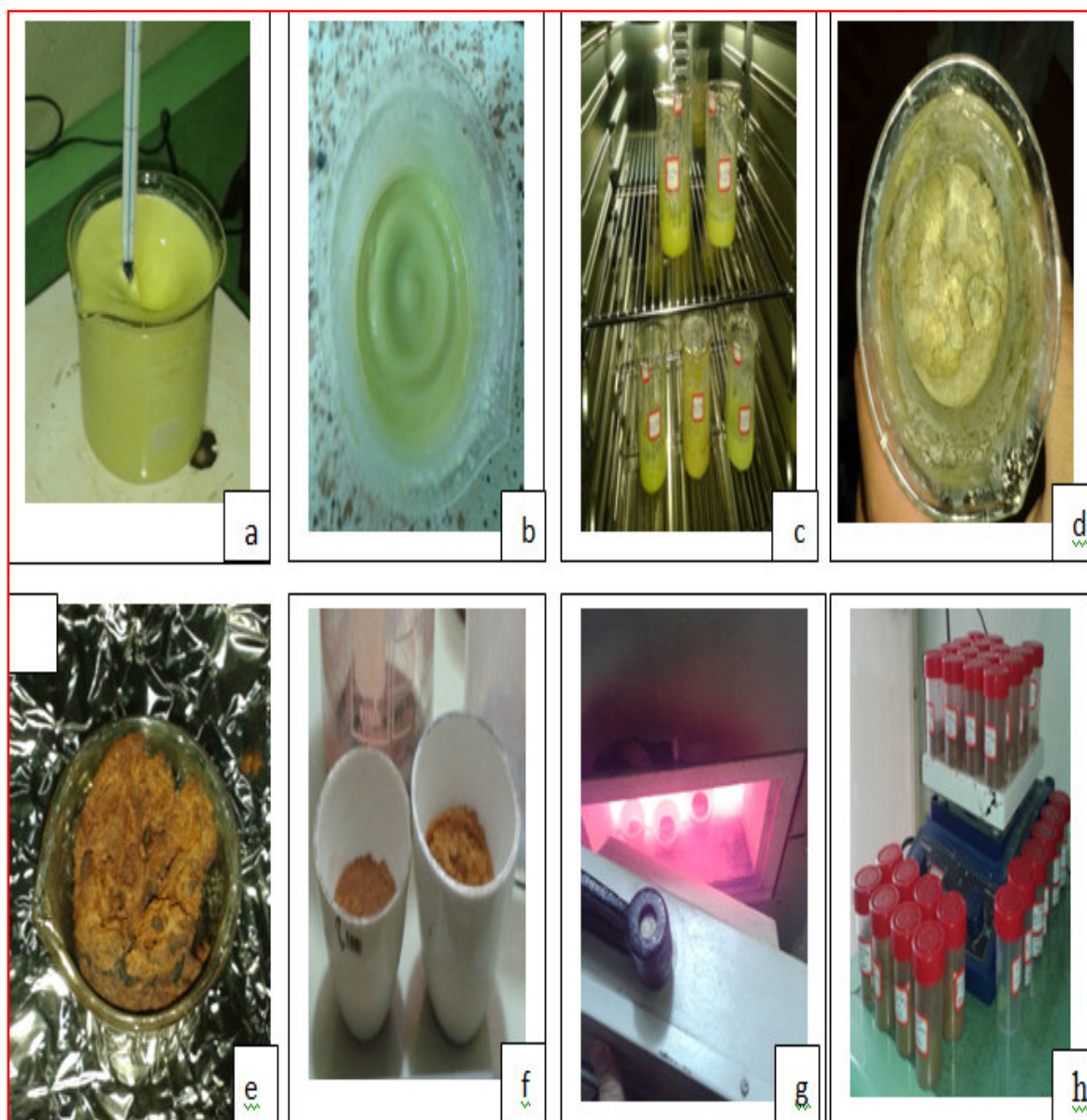
Figure (3-1) Photograph of (a) The solution after the adding of ammonia, (b) the gel, (c) gel in oven to dry, (d) ) dry gel, (e) auto combustion and become nanopowders ferrite (f) nano powder, (g) nano powder at different temperature, and (h) calcinated in the oven at 250°C, 400°C, and 600°C .
