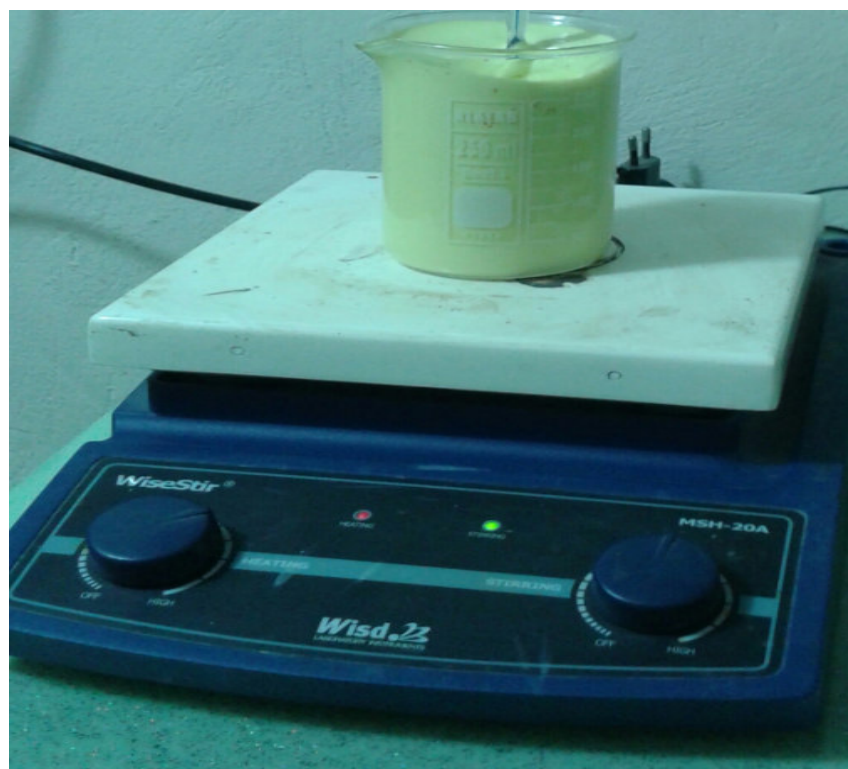
Figure (3-10) Magnetic Stirrer
